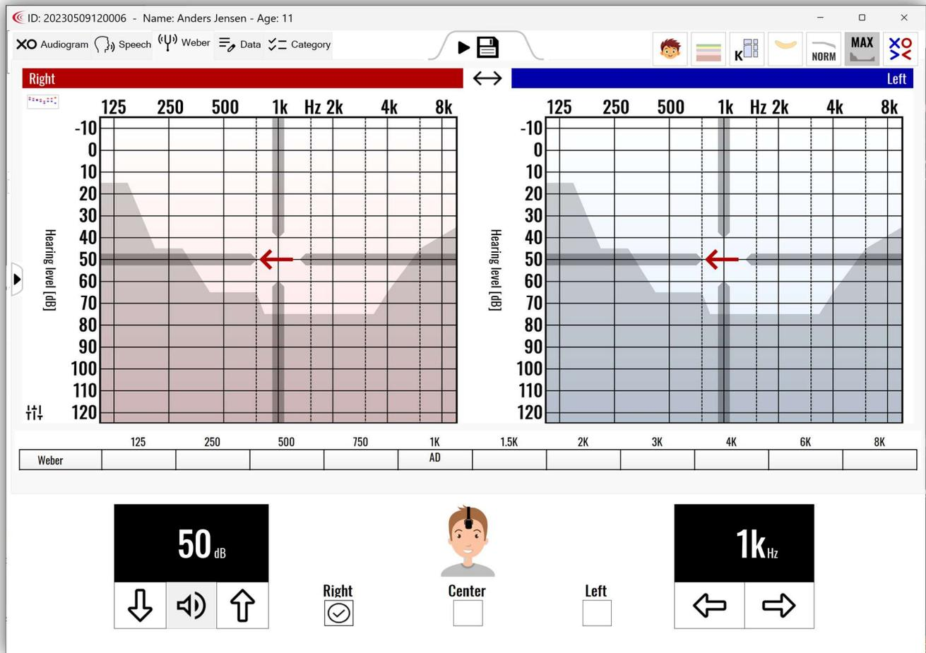
1. Adjust the dB hearing level and the frequency if needed.
