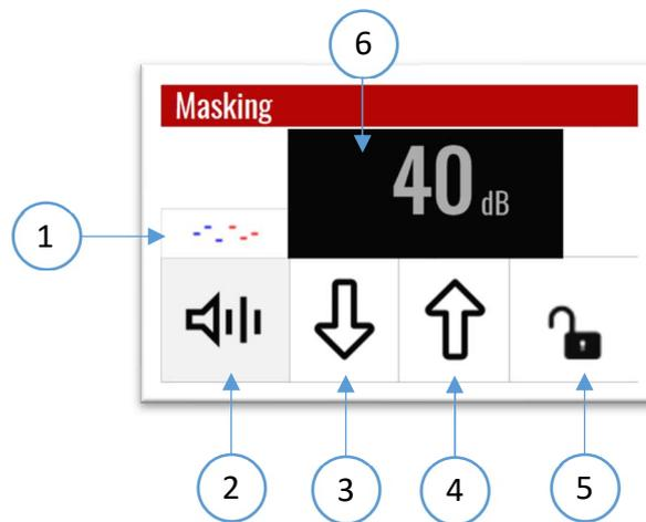
1. Toggle common/separated masking – Set masking levels for each frequency
